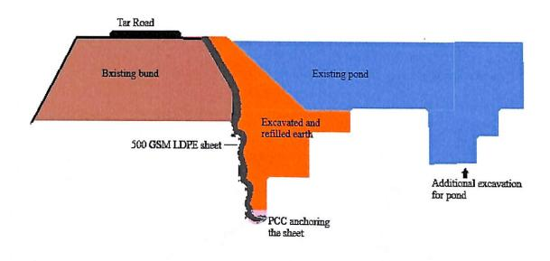
Schematic section of the Sub-Surface dyke (not to scale)
