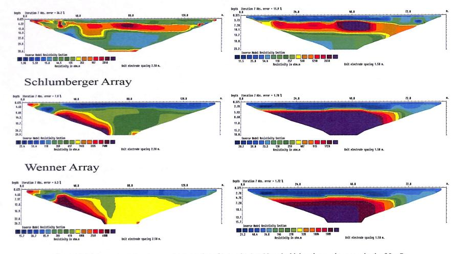
Figure: 14 2D images in different arrays at a separation of 2.5 and 1.5 m. Note the high resistance layer at a depth of 5m-7m
