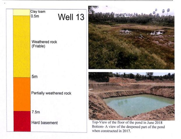
Pond overflowed on 23.07.2018. The over flow continued from the pond and peaked on 16.08.2018 when the water level above the over flow point (cemented steps) was 1.5 m. Over flow from the pond continued till the middle of November, 2018. On 30.08.2018, the water level stood at 0.4 m above the overflow point while it was 0.3 m on 14.10.2018.
