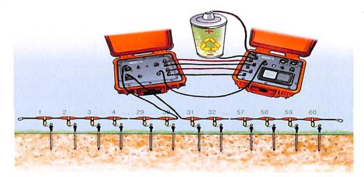
Figure 12: Survey Layout sketch for 2D ERT of WGMD-4 Model
