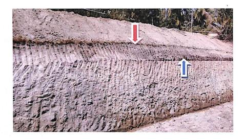
Figure: 17a. Photograph showing the upper cross section of the trench. The red arrow above points to the dark line indicating present floor of the pond. The horizontal dark line indicated by blue arrow below shows a 75 cm thick clay deposit above the original pond floor that accumulated over a period of time. In the extreme bottom of the excavation weathered rock is starts appearing.
