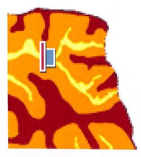
Figure.8: Upper part of Ozhalapathy watershed in the Kerala side is given in the figure on the left. Dark red shows the elevated parts, yellow are the valley and orange depicts side slopes. The runoff from the two valley portions are collected in the pond (blue rectangle). The bund on the lower part is shown in red.
