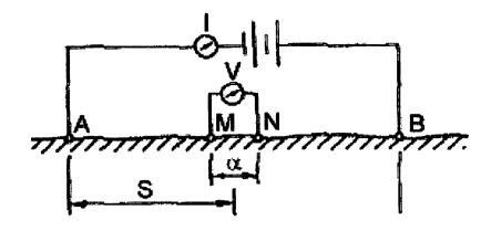
Figure 11a: Schlumberger array configuration
