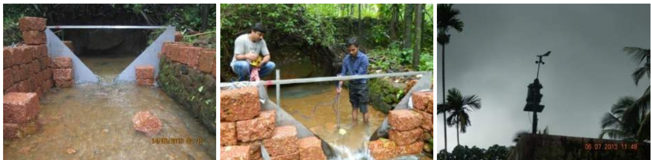
a. Discharge flow measuring from V-notch wire b. Rainfall- Automatic weather station
