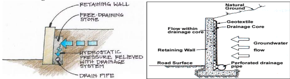
Figure 7.6 Typical section of retaining walls suitable for stabilisation of lateritic railway cutting prone to soil piping (Panjami 2016)
